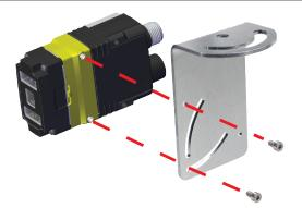
Align the holes on the mounting surface with the mounting holes on the vision system. Insert the M3X3.5 screws into the mounting holes.
