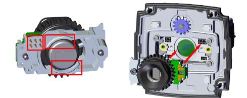
b. Tighten the M2 x 5 mm HSH screw halfway, then tighten the M2 x 12 mm HSH screw halfway as well. Continue screwing each screw incrementally, until tightening them to 0.4 Nm, using a torque wrench.
