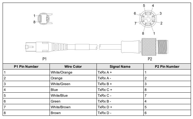
**CAUTION**: The Ethernet cable shield has to be grounded at the far end. Whatever this cable is plugged into (typically a switch or router) should have a grounded Ethernet connector. A digital voltmeter has to be used to validate the grounding. If the far end device is not grounded, a ground wire should be added in compliance with local electrical codes.
